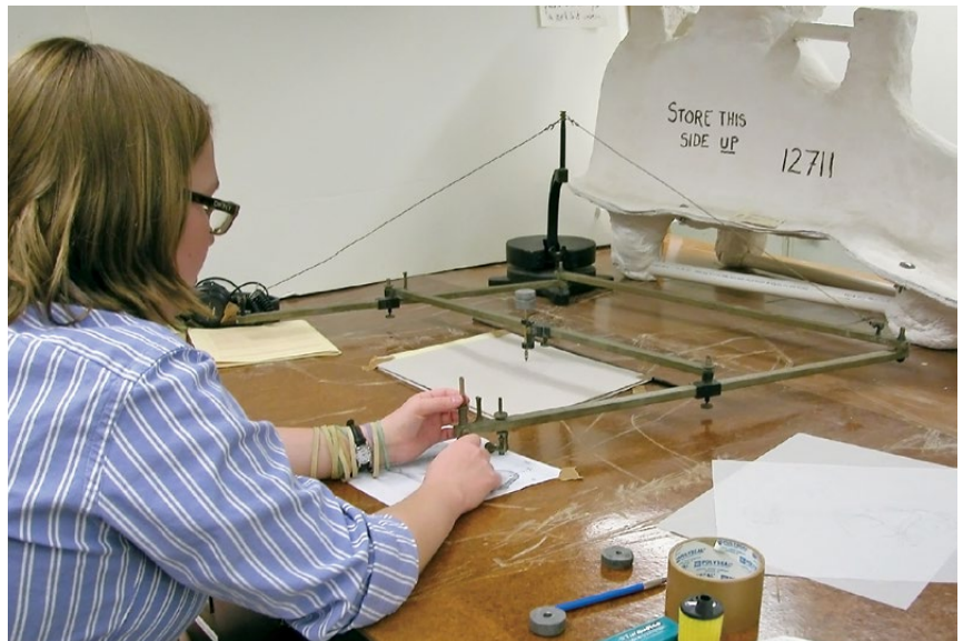
Figure 6: Julia Coursey using the pantograph to trace and resize a drawing. Photo by Mary Parrish.
